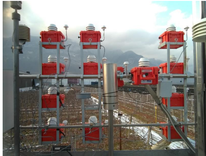
Figure 13: Intercalibration of innovative air quality sensor at roadside AQ station at km 103.
