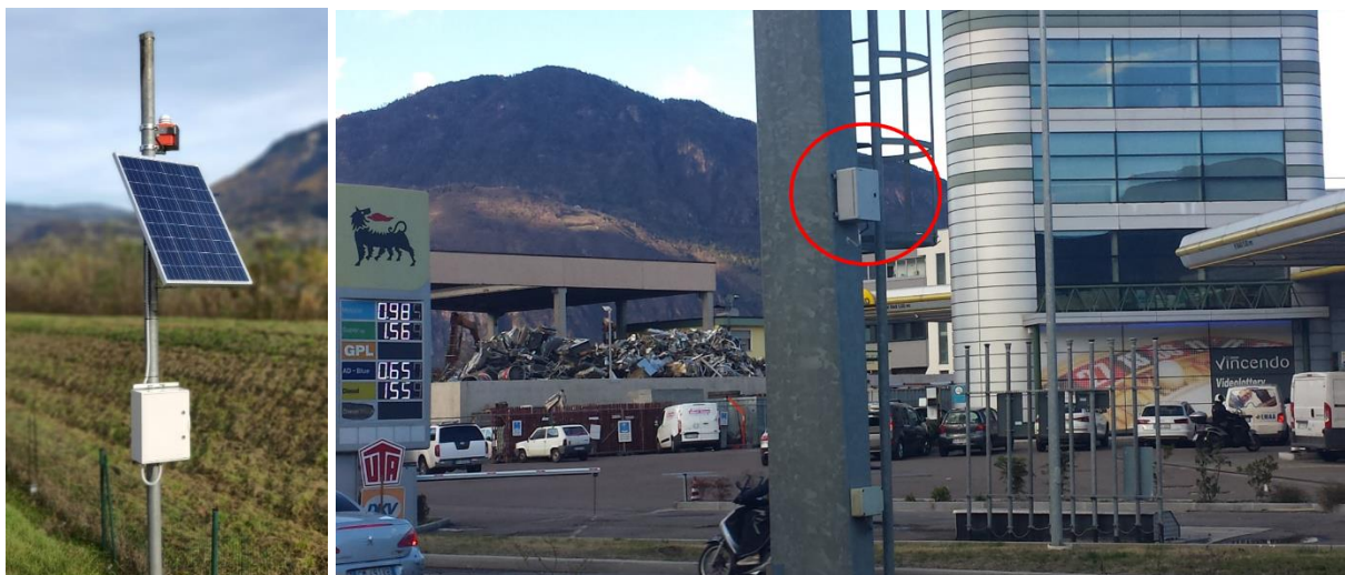
Figure 2: Low-cost air quality sensor (on the left) and Bluetooth sensor (on the right).
